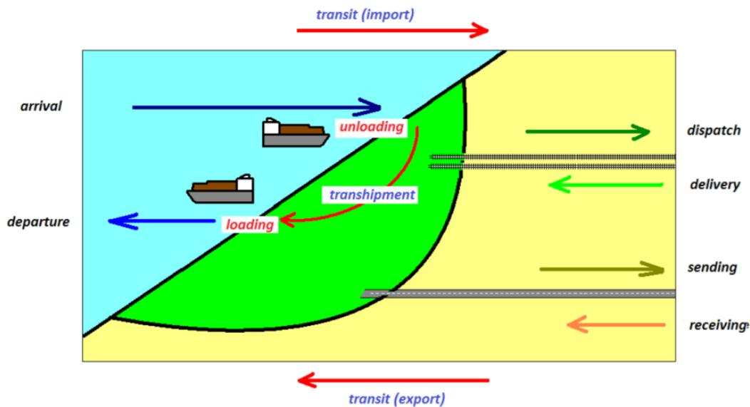
Fig. 2. Port as a node of cargo flows
