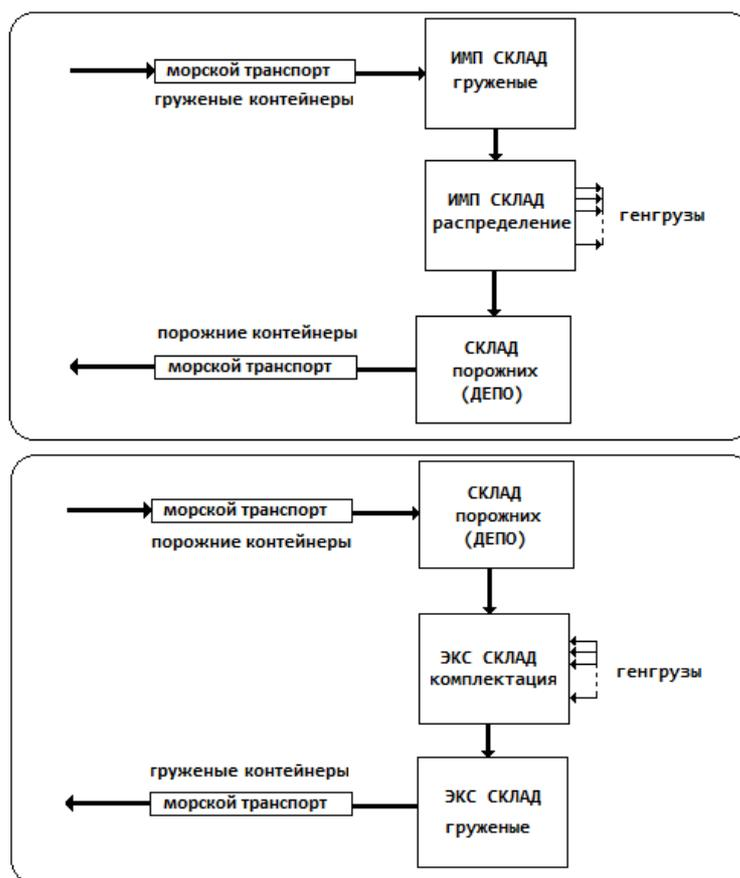
*Fig. 131. Functional models of industrial container port*
