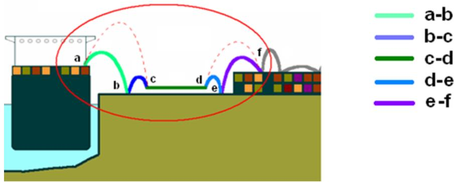
Fig. 17. Transportation Sea-CY broken into primary moves
