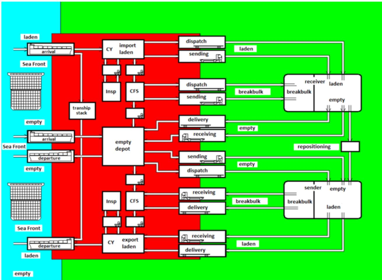
*Fig. 8. General functional model of container terminal*
