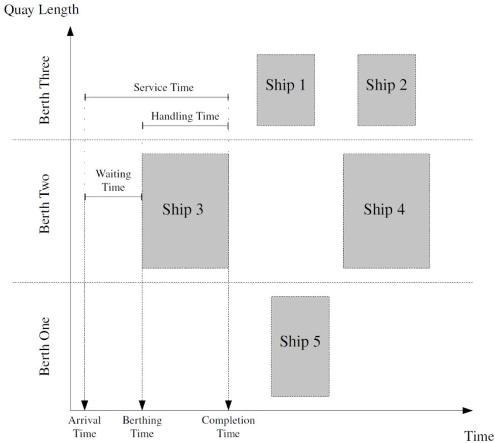
*Fig. 1 The representation of the berth-time space*
