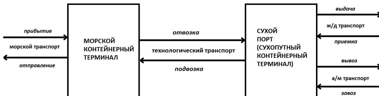
*Fig. 4. Interaction of sea and hinterland terminals*
