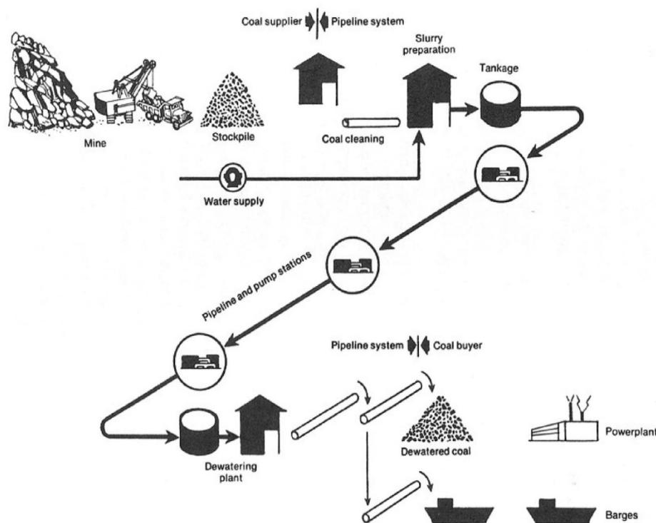
*Fig. 1. Schematic flow diagram for a one-way water coal slurry pipeline [7]*
