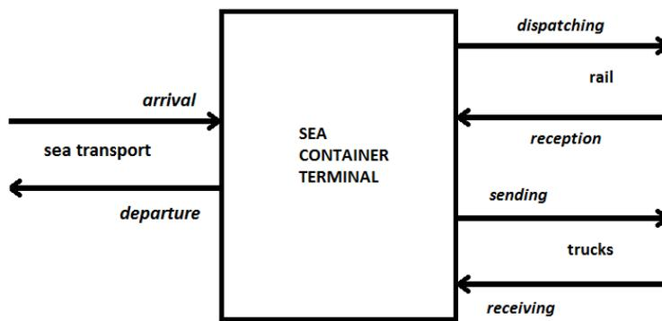
Fig. 2. Operations of the sea container terminal
