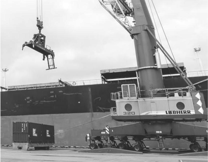
*Fig. 2 – Cargo transshipment out of the containers on to the vessel*
