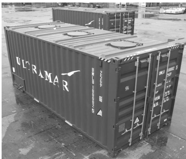
*Fig. 1 – The specialized bulk container for the transfer and storage of bulk cargoes*
